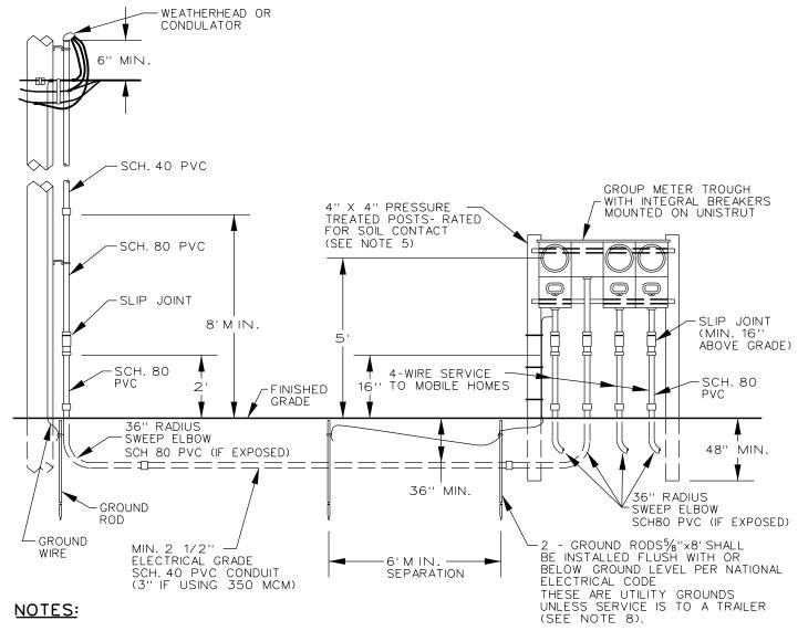
1. THE LOCATION OF THE PEDESTAL WILL BE DESIGNATED BY A UTILITY REPRESENTATIVE. THERE SHALL BE NO MORE THAN 3 NINETY-DEGREE BENDS IN THE CONDUIT, INCLUDING ONE AT THE POLE/PAD AND ANOTHER THE PEDESTAL.
