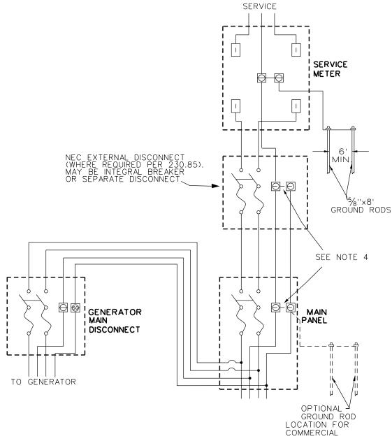
THE GENERATOR MAIN DISCONNECT SHALL BE LOCATED WITHIN TEN FEET OF, AND IN VIEW OF, THE SERVICE METER OR THERE SHALL BE A PLACARD WITH DIRECTIONS TO THE DISCONNECT PER NEC.
